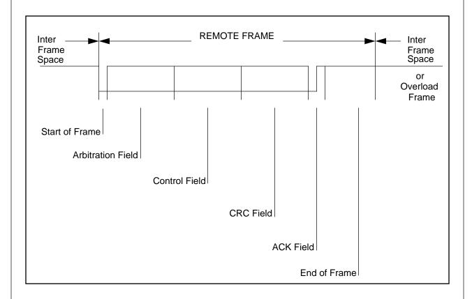
The polarity of the RTR bit indicates whether a transmitted frame is a DATA FRAME (RTR bit 'dominant') or a REMOTE FRAME (RTR bit 'recessive').
