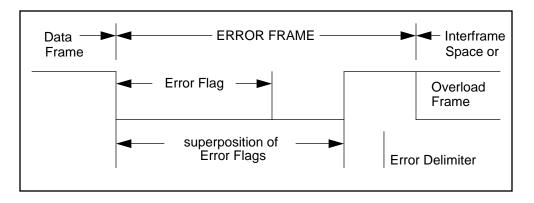
In order to terminate an ERROR FRAME correctly, an 'error passive' node may need the bus to be 'bus idle' for at least 3 bit times (if there is a local error at an 'error passive' receiver). Therefore the bus should not be loaded to 100%.
